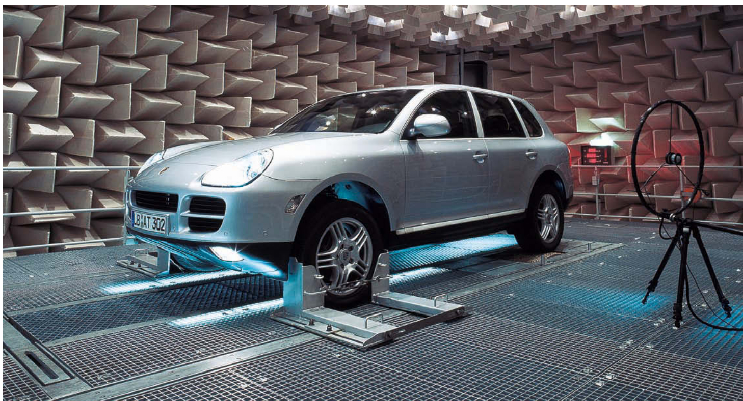
Below and right: Porsche's acoustic chambers measure engine, drivetrain and component sound Above: The sound symposer system from the Cayenne GTS pipes noise into the cabin to augment the driving experience
